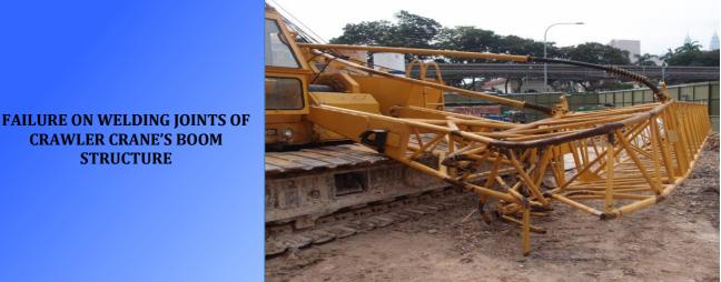
An accident involving a crawler crane had occurred during dredging activity for pile casing installation. The pile casing was installed using vibro-hammer that has been suspended on the main hook block. During the accident occurred, the crane operator has shifted the crane boom position from falling outside the construction area after it's started to fail. No casualty was reported from this accident.
