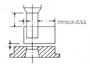
WHERE FIXED EJECTOR PLATES ARE FITTED A GUARD NEED NOT BE PROVIDED UNLESS THE DISTANCE "E" EXCEED 3/16" IN WHICH CASE THE TOOL MUST BE PROVIDED WITH A GUARD AS SHOWN
