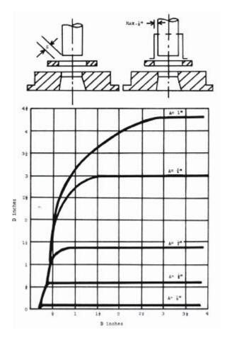
The distances "A" & "B" are determined by the form and size of the work. The distance "D" can be determined by reference to the graph.
