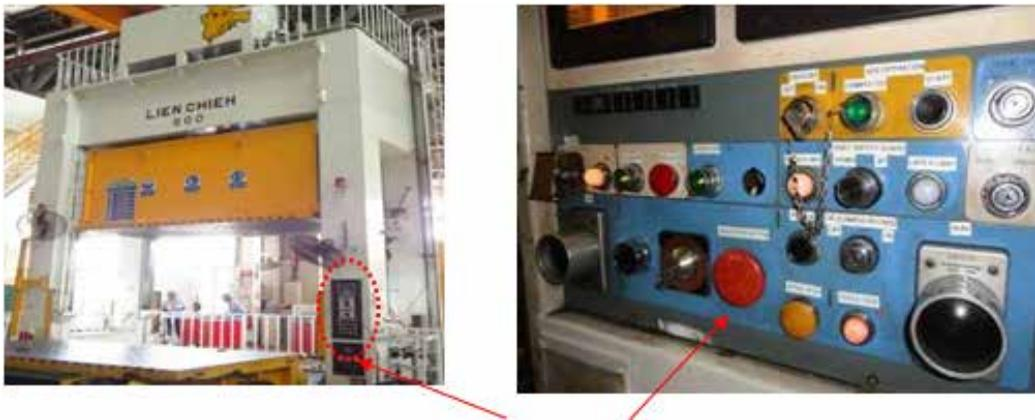
**Figure 26 Location Of Emergency Stop At Control Panel**
