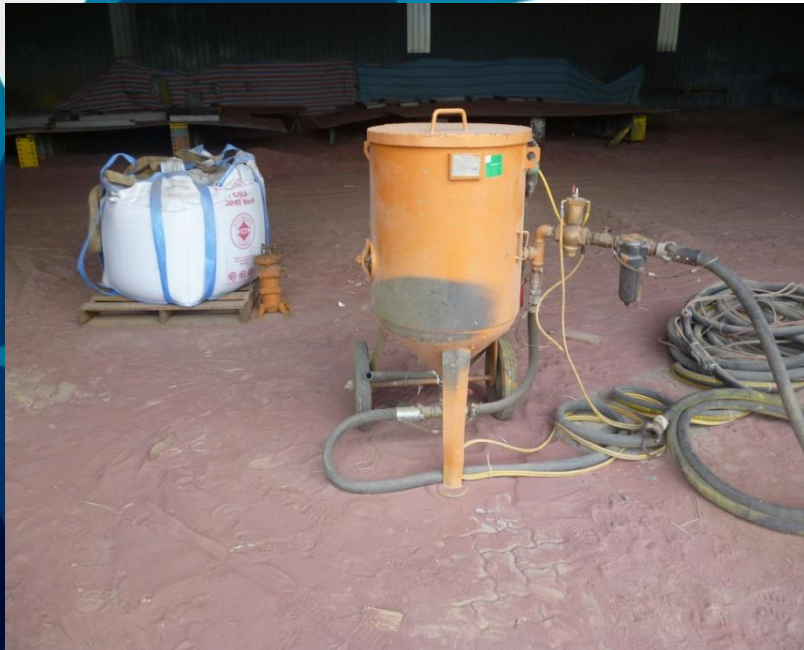
Blasting Pot at Blasting Chamber Medium used : Garnet
