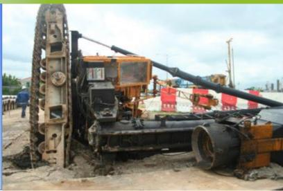
An accident involving piling rig machinery occurred at a construction site recently. The incident occurred when the piling rig operator was lifting a piece of steel plate to be used as a base of the machine for piling works to be carried out at the site.
