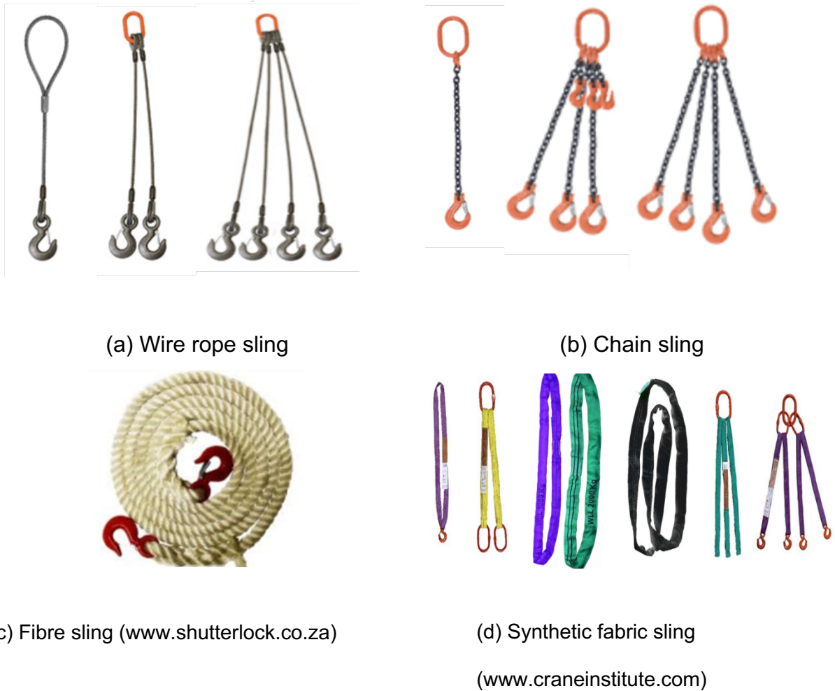
Figure 3.24 Types of slings that are usually used at construction sites ( www.uscargocontrol.com/Lifting-Slings )
