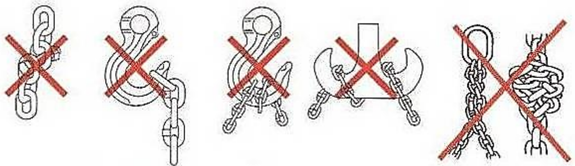
Figure 3.21 Wrong ways of using chains ( www.practicalmaintenance.net )
