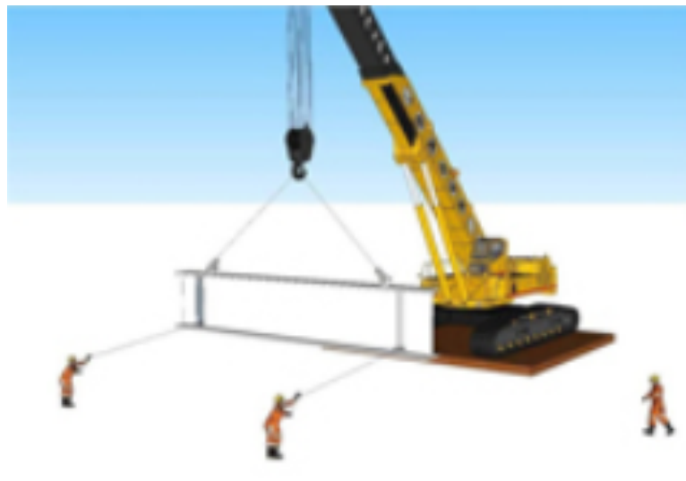
Rajah 3.23 Use more than one of fibre ropes to control loads ( www.cranetech.com )
