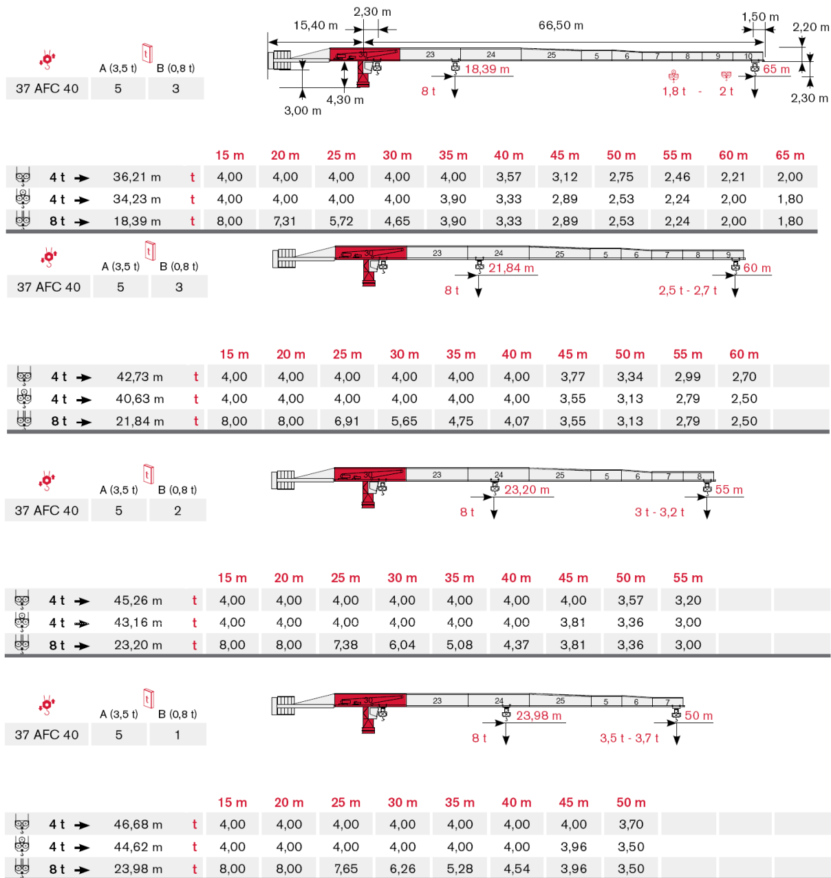
Figure 4.8 Example of load chart for topless hammerhead tower crane (www.bigge.com)
