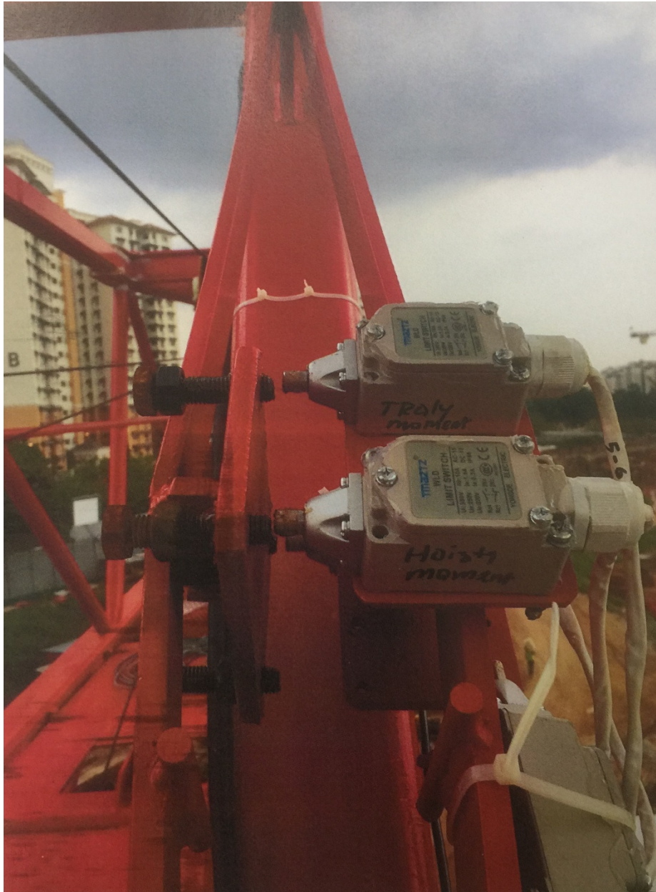
Figure 7.6 The limiting switch attached to the A-frame tower crane
