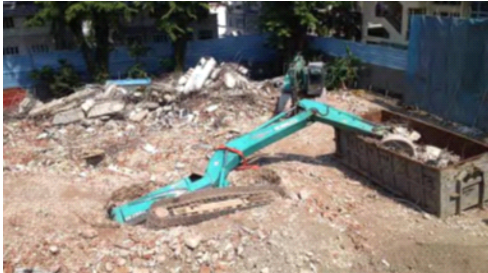
Figure 5.1 Machinery that sink in dense ground areas ( Ground Conditions for Construction Plant Strategic Forum for Construction, Good Practice Guide, London, 2014 )
