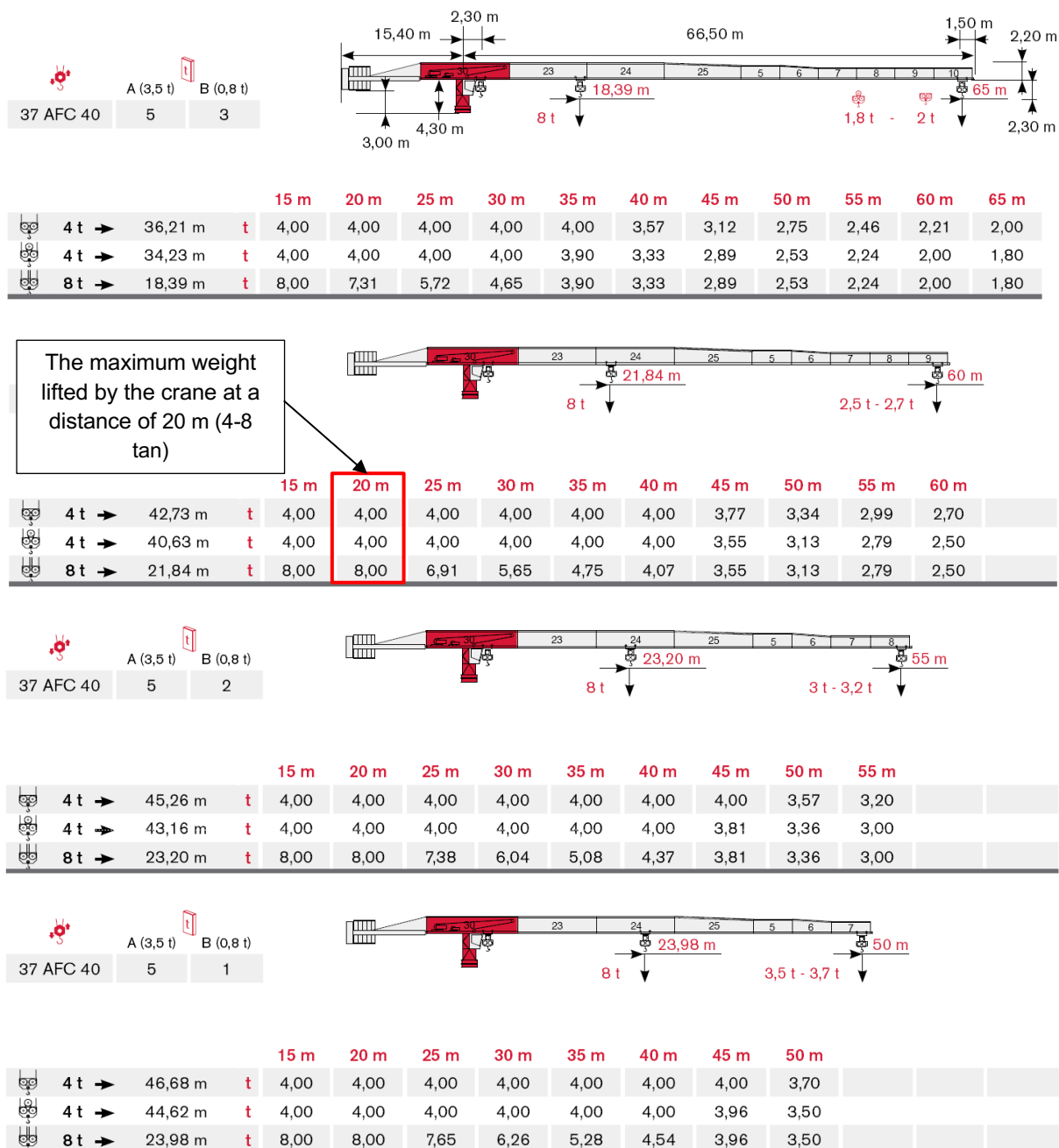
Figure 5.8 Load chart for topless hammerhead tower crane (www.bigge.com)
