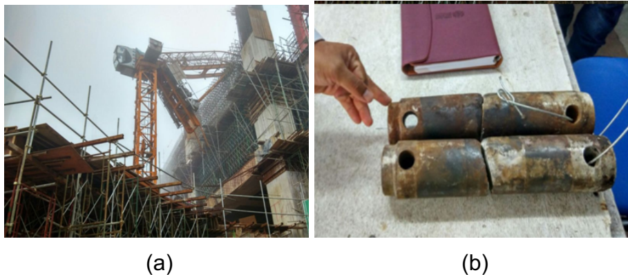
Figure 4.13 Failure of tower crane in Kuala Lumpur 2016 (a) Overluffing crane and (b) broken connection pin ( http://www.dosh.gov.my )
