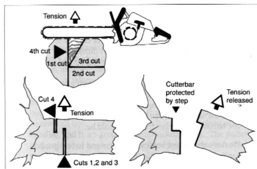
**Figure 14: butting a tree under tension**
