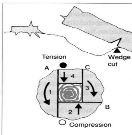
Figure 16: Crosscutting o log under suspension
