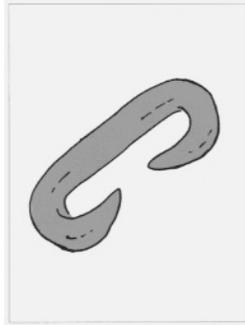
2.7.1.8 “C” type hooks of the type illustrated in figure 1 shall not be used in any logging operation.
