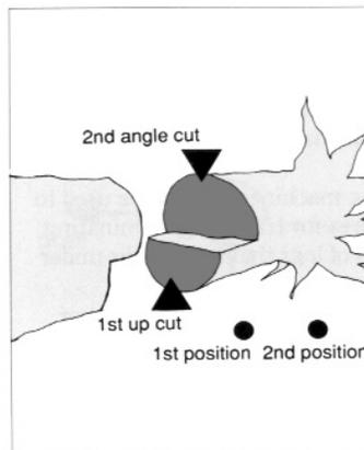
**Figure 13: Butting off a tree that may spring upwards and sideways**
