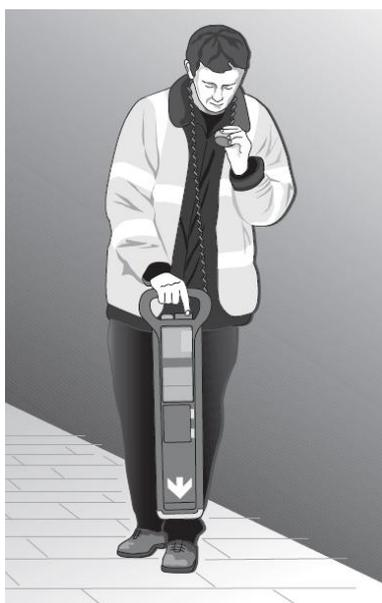
Figure 18. Using a cable locator by properly trained people to identify as far as possible the actual location of underground services (Hughes, et al., 2008).
