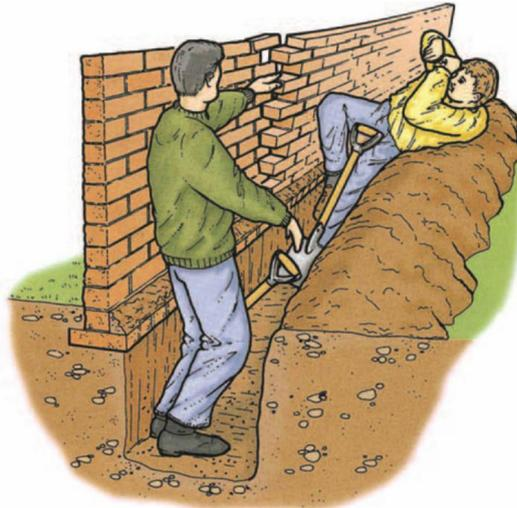
Figure 2. Stability of structures adjoining or over areas to be excavated must be protected (Hughes, et al., 2008). Where there is any question of stability of structures adjoining or over areas to be excavated, such structures shall be supported where necessary by underpinning, sheet piling, shoring, bracing or other means made or erected according to the design of a Professional Engineer to prevent injury to any person (FMA, 2014).
