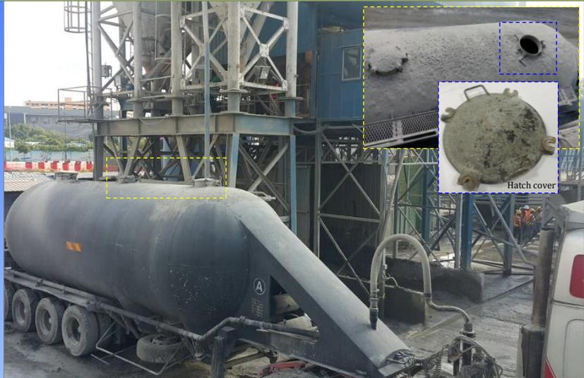
A cement tanker driver/operator sustain injury after one of the hatch covers positioned on top of the tanker detached and struck him. The impact pushed him down from the tanker. Shortly before the incident, the victim was doing some adjustment at the respective hatch cover.
