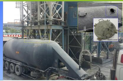
A cement tanker driver/operator sustain injury after one of the hatch covers positioned on top of the tanker detached and struck him. The impact pushed him down from the tanker. Shortly before the incident, the victim was doing some adjustment at the respective hatch cover.
