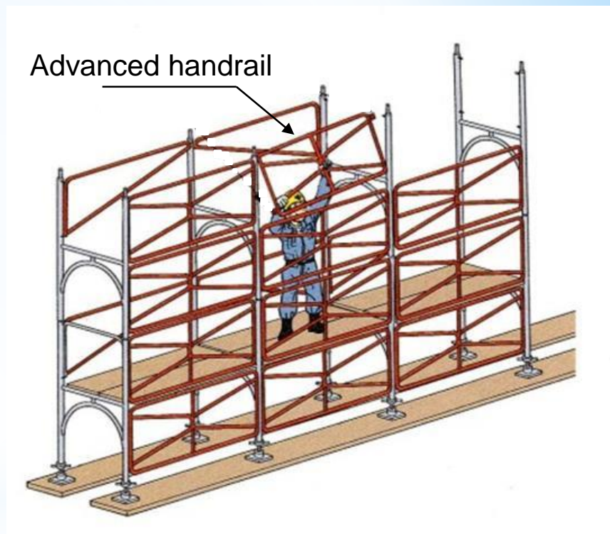
Method to erect handrails first using special scaffolding
