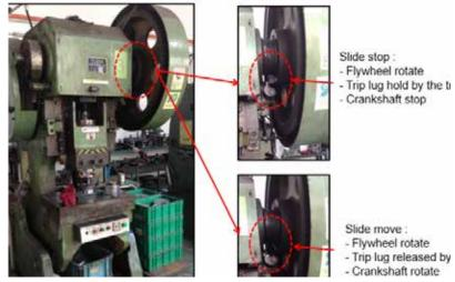
Figure 2 Full-Revolution Clutches
