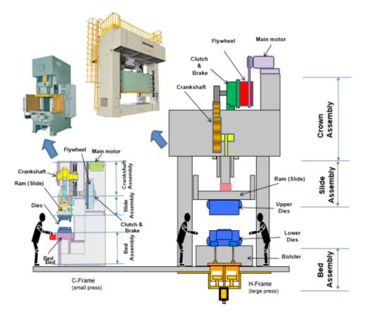
Figure. 1 Mechanical Press
