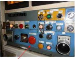
Figure 26 Location Of Emergency Stop At Control Panel
