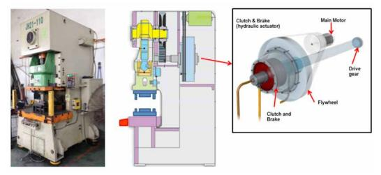
Figure 4 Part-Revolution Clutches
