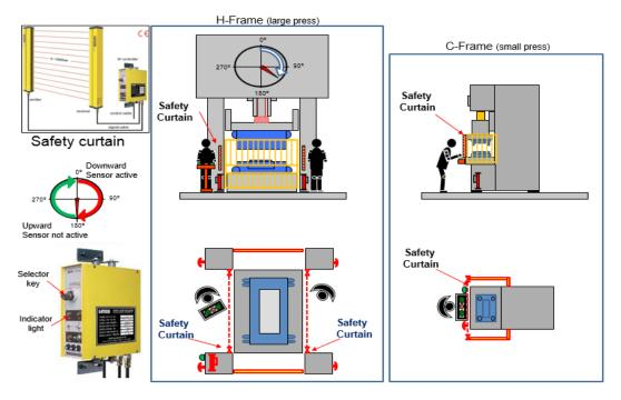
Figure 21 Safety Light Curtain sensor
