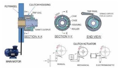
Figure 3 Simplified Cross Section of Full-revolution clutches
