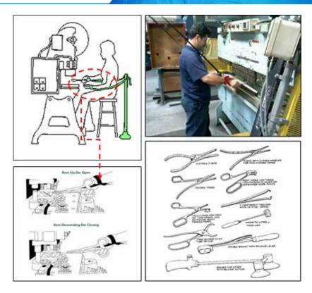
Figure 13 Restraint Device With Hand Feeding Tool
