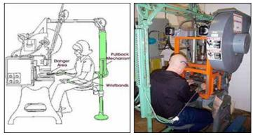
Figure 14 Pullback Devices
