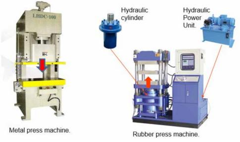
Figure . 7 Hydraulic Power Unit
