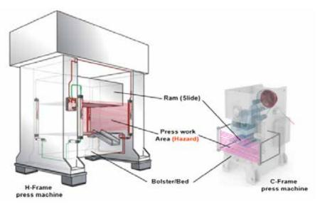
Figure. 9 Hazard area (Point of Operation)
