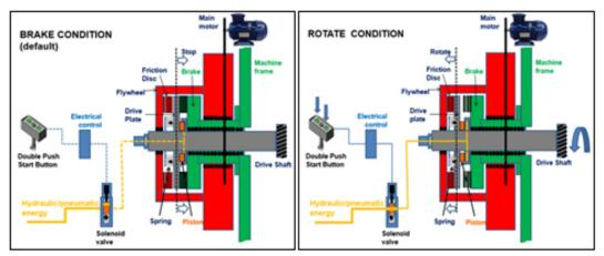
Figure 5. Simplified Cross Section of Part-revolution clutches
