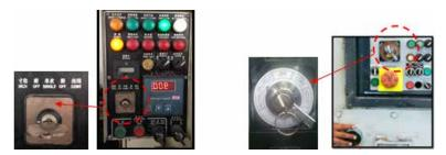
Figure 17 Operation Selector Switch
