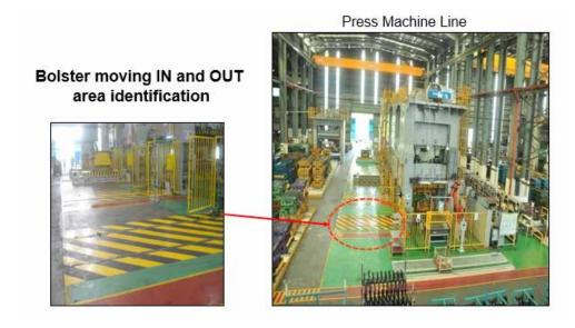
Figure 28 Marked Area For Moving In And Out Of Bolster
