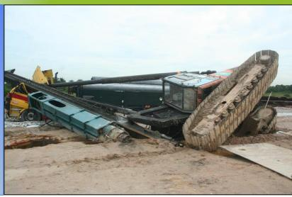
An accident involving a piling machinery occurred at a construction site recently. The piling machinery toppled while it was moving and had crashed a nearby truck. This incident resulted in severe damage to the prime mover of the truck and the lorry driver was injured in the head.
