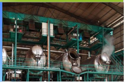
An explosion occurred in the sterilizer causing the inlet quick opening door in the sterilizer forced open around 12.30 pm. A complete cycle of a fresh fruit bunches (FFB) cooking process occurs at 42 psi steam pressure for 50-52 minutes. During the event, the sterilizer unit was found to explode at 30 psi steam pressure resulting the inlet quick opening door of the sterilizer forced open from inside. The contents were thrown out and caused damage to the part of the building's wall structure.
