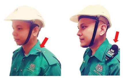
Figure 7.2: Position of microphone.
