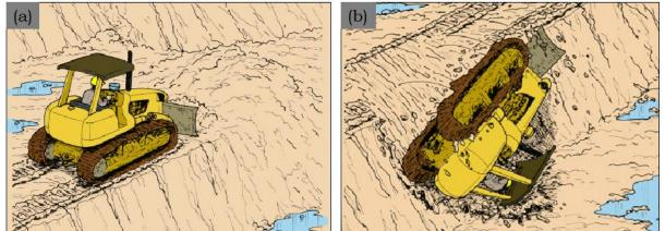
Figure 21. The excavation and its vicinity must be inspected by a designated person after rainstorm (JICOSH, 2015).
