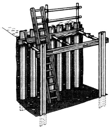
Figure 5. In open sheeting, the sheets are only placed at intervals (HSE, 1999).
