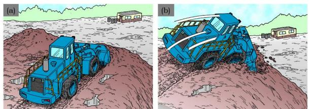
Figure 8. Operating the vehicle at the edge of the bank can cause the edge of bank to collapse (JICOSH, 2015).
