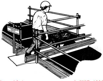
Figure 16. Access-way across trench (HSE, 1999).
