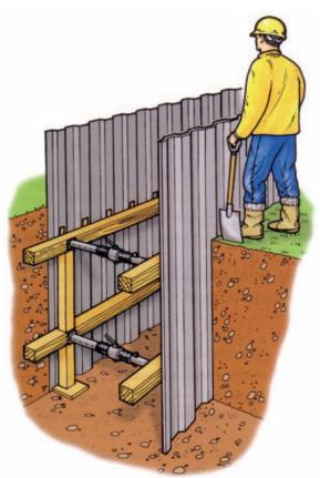
Figure 4. Trench sheets with timber walings, screw props, puncheons and sole plates (Hughes, et al., 2008). Timber packing should be used to prevent struts bearing directly on steel.
