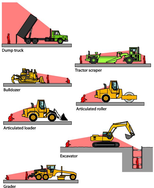
Figure 14. Mobile plant operator blind spots. Powered mobile plant operating near ground personnel or other powered mobile plant should be equipped with warning devices (for example, reversing alarm and a revolving light) (SafeWork, 2012).
