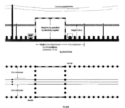
Figure 20. Diagram showing normal dimensions for 'goal post' crossing points and barriers (HSE, 1999).
