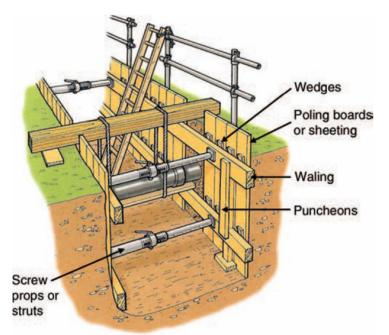
Figure 3. Timbered excavation with ladder access and supported services (guard removed on one side for clarity) (Hughes, et al., 2008). Underground services which are exposed by the excavation are supported.
