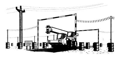
Figure 19. Precautions for overhead lines: 'goal post' crossing points beneath lines to avoid contact by plant (HSE, 1999).
