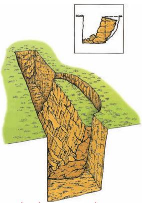
Figure 1. All practicable steps must be taken to prevent danger to any person in and adjacent to the excavation, to ensure that no excavation or part of it collapses (Hughes, et al., 2008).
