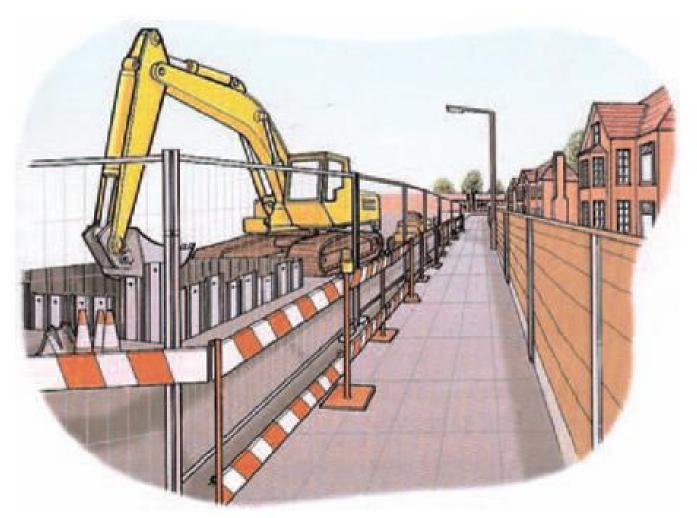
Figure 15. All public walkways, sidewalks, and the thoroughfares bordering on or running through any excavation site shall be provided with substantial guard-rails or board fences. Barriers around excavation by footpath (Hughes & Ferret, 2008).
