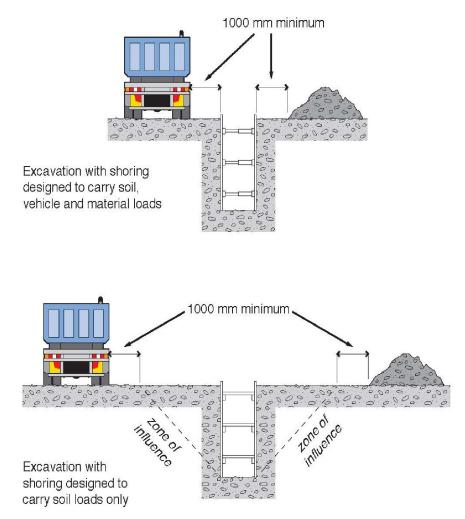
Figure 11. Mechanical plant, vehicles, storage of materials (including excavated material) or any other heavy loads should not be located in the 'zone of influence' of an excavation (SafeWork, 2012).
