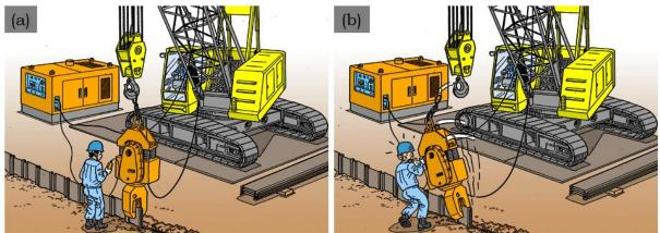
Figure 6. Removing sheet piling using the vibrohammer without securing the hydraulic chuck may cause the vibrohammer to come off its hook and fell onto the worker (JICOSH, 2015).
