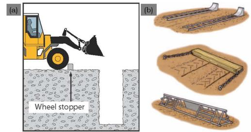
Figure 10. Adequate and well-anchored stop blocks should be provided on the surface to prevent vehicles being driven into the trench, cofferdam or caisson (a). Examples of stop blocks for dumpers (b) (Hughes, et al., 2008).
