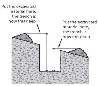
Figure 17. Excavated material impact on effective excavation depth (SafeWork, 2012).
