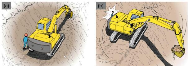
Figure 9. No employee shall be permitted to work where he may be struck by an excavating machine. Put up a barricade to prevent entry and assign a supervisor to the construction site (JICOSH, 2015).
