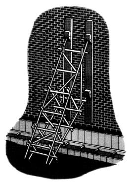
Figure 7. Shoring of building with excavation at base. Care should be taken to ensure that the foundations of nearby buildings or structures are not disturbed or undermined (HSE, 1999).
