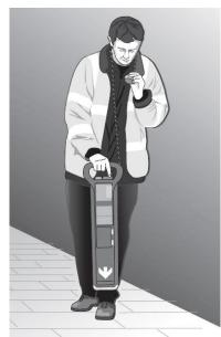
Figure 18. Using a cable locator by properly trained people to identify as far as possible the actual location of underground services (Hughes, et al., 2008).
